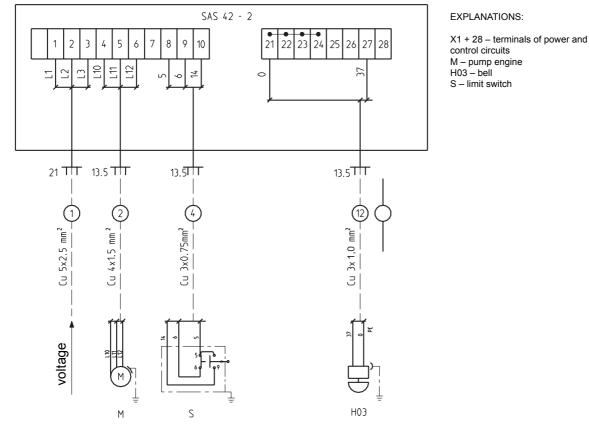
Fig. 4 Wiring diagram of control unit SAS 42-2
