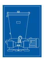
20, 32, 40 MPa 1,1 kW 230/400 V or 3x500 V plastic grease of the consistence class  $\leq 2$ acc. to PN/72 C-04095 (NLGI) -10 ... 60°C 70 dm<sup>3</sup>
