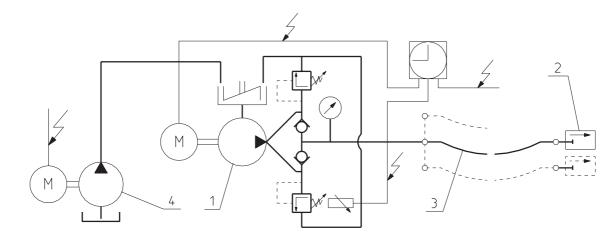
Fig. 5 Constructional diagram of equipment of lubrication stands in vehicle and machine service stations
