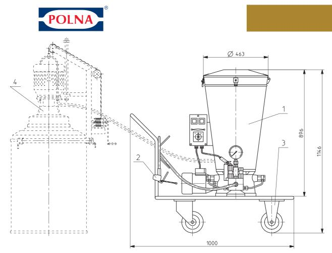
Fig. 2 Overall dimensions of the lubrication stand SA 1
