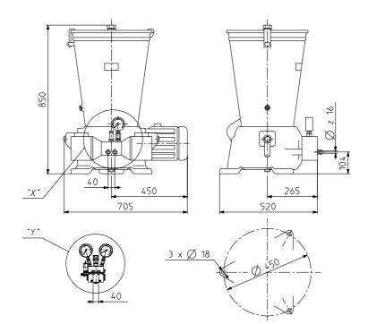
Fig. 3 Overall and linkage dimensions of the pump
