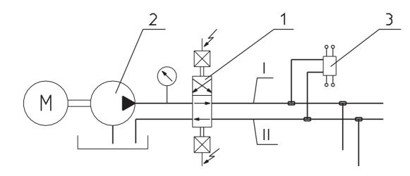
Fig. 1 Scheme of a lubrication system with the electromagnetic distributor 1 - Distributor, 2 - Pump, 3 - Feeders, I - II - Iubrication main conduit lines
