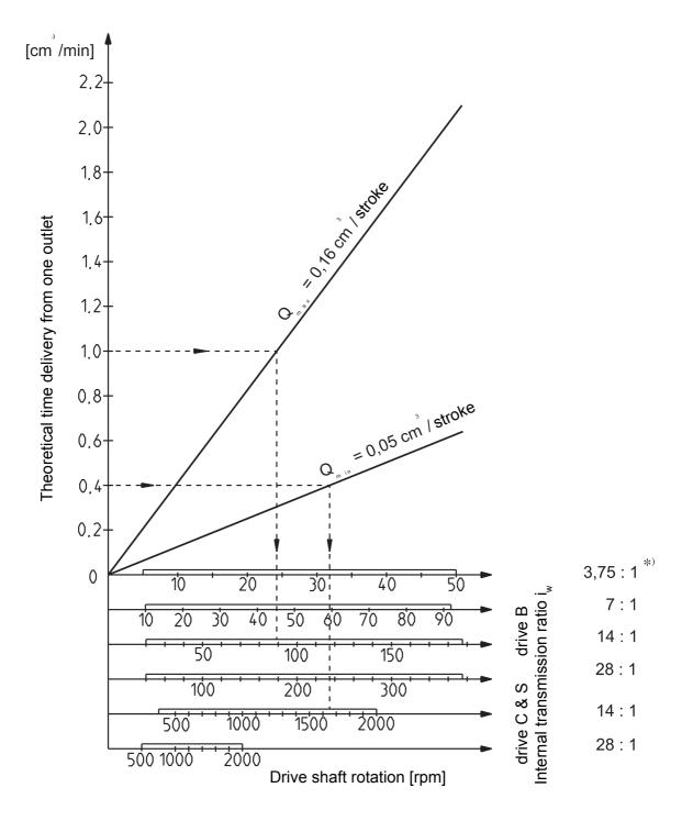
Fig. 3 Diagram of time delivery of pumps MPS 10-2 type, with drive B, C, S
