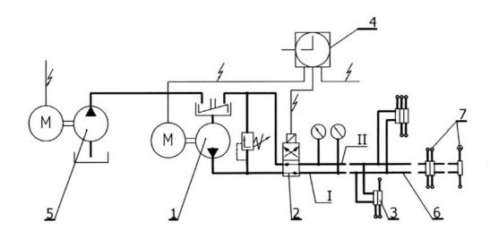
Fig. 1 Construction diagram of the two-way force feed oiling systems
