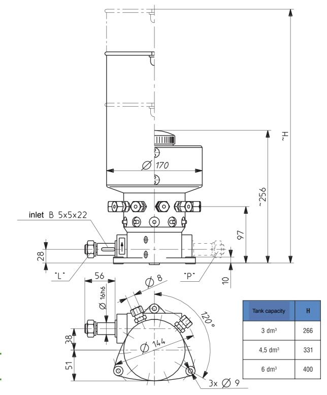
Fig. 5 Grease and oil lubrication pump with rotary drive of MPS 10-B type
