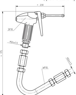
Fig. 1 Overall and linkage dimensions
