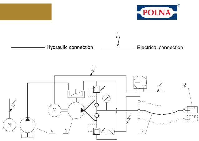
Fig. 4 Construction and operational scheme of the lubrication stand
