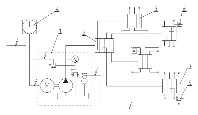
Fig. 3 Example scheme of a progressive force feed oiling systems
