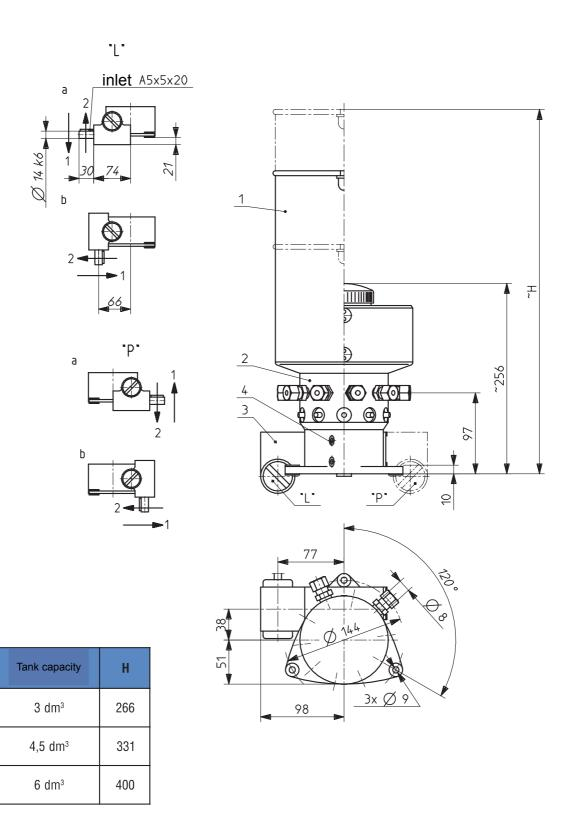
Fig. 6 Grease and oil lubrication pump with drive and additional reduction gear of MPS 10-C type
