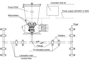
Fig. 2 Construction diagram of the central lubrication system with a PD 30 pump
