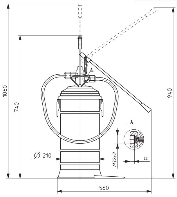
Fig. 1 Dimensions of the pump
