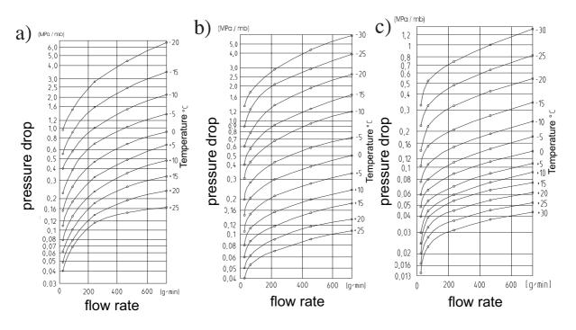
Fig. 2 Diagrams of pressure drops at forcing plastic grease IP1-Z through pipes of nominal diameters: a=9 mm; b=13 mm; c=25 mm.
